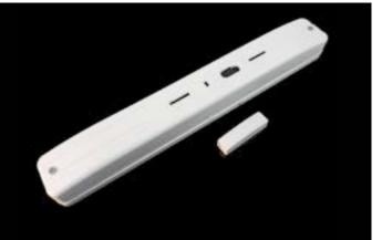
The dual IR perimeter detector allows monitoring access points using two different detection methods. Two IR sensors allow monitoring free entry points like windows or balcony doors. The unit's linear lenses create a curtain detection area. Operation in AND with a 24 Ghz microwave ensure high immunity to false alarms.
